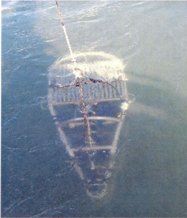
Figure 13: ZAPS instrument package being towed in the Columbia River Estuary. Photo courtesy G. Klinkhammer, COAS, Oregon State University.
