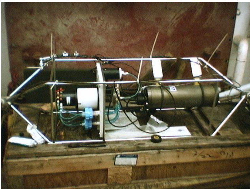
Figure 16: This particle collection system filters water for selected periods of time, thereby allowing in situ collection of particles from large volumes of seawater. An electric pump passes water through membrane cartridges that can be recovered once the system is brought back to the surface.
