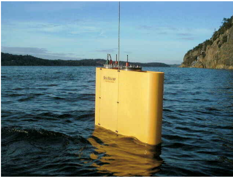
Figure 3: Sea Tramp autonomous, multicycling, data collecting platform designed for unattended marine monitoring and research. It profiles along a guiding wire and performs well also in stratified waters and when equipped with non stream-line payload. Sensors are selected by the operator and may be installed on site.
