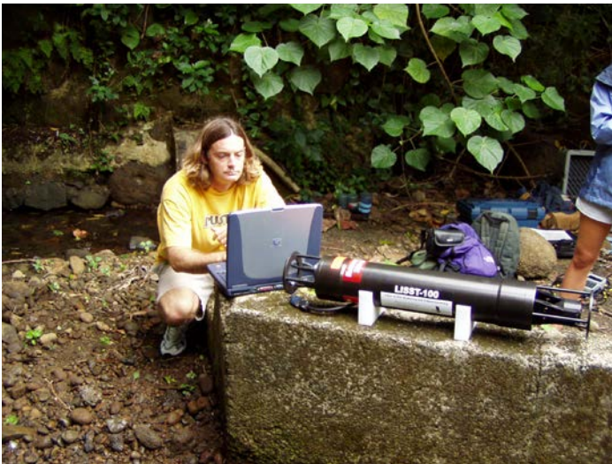
Figure 19: LISST 100 instrument undergoing programming by graduate student, C.W. Young, prior to deployment in Waiakeakua Stream, Oahu, Hawaii.
