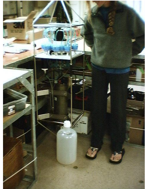
Figure 15 (right): Mc Lane Particle collector system used aboard R/V Roger R. Revelle during EPREX 2000 cruise.
