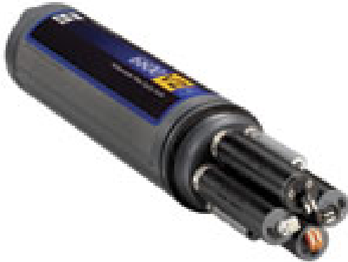
Figure 2: Profile of the new 6600 EDS depicting probes for temperature-conductivity (small probe), chlorophyll, turbidity, ROX (optical) dissolved oxygen, and pH/ORP. Probes are maintained free of fouling by the Clean Sweep™ universal wiper assembly, as well as individual optical wipers. (Conductivity is not cleaned by the wiper).
