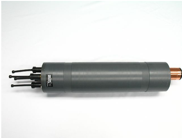
Figure 11: The ISUS V3 nitrate sensor is a real time, chemical free system designed to overcome the traditional challenges associated with reagent-based nitrate analysis. The ISUS technology uses advanced UV absorption technology to provide accurate nitrate concentration measurements.
