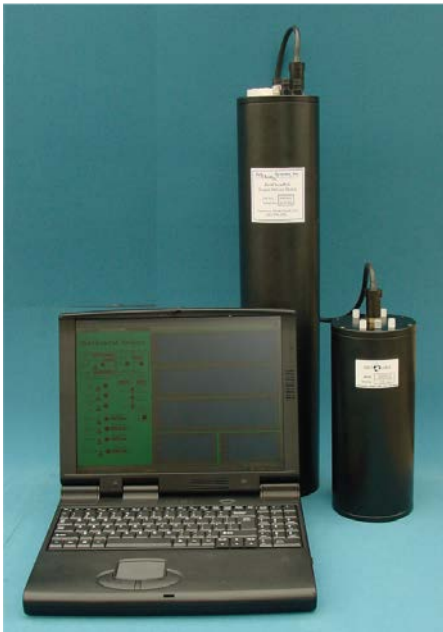
Figure 6: (left) SubChem Pak Analyzer and battery.
