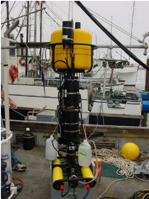
Figure 8: SubChem Systems APNA system for shipboard profiling applications. Components are shown below: Left: exposed analyzer, right: Analyzer and battery pack
