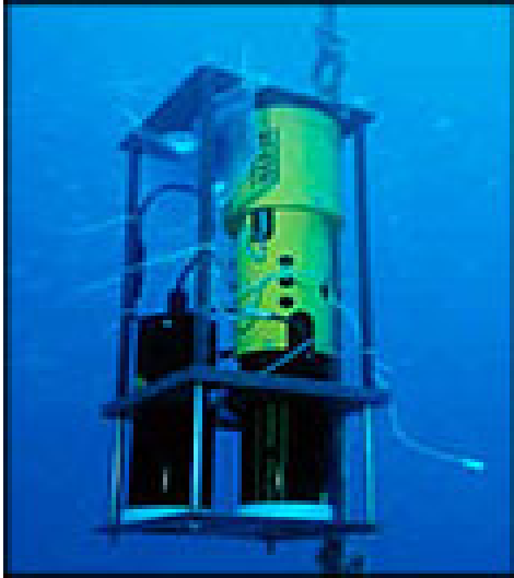
Figure 10: NAS-2E system deployed on a mooring. Note the main (yellow) instrument control box and the two (black) cylindrical analyzers for N and P analysis. The NAS systems are capable of determining nitrate (and/or nitrite) phosphate, silicate, and ammonia.
